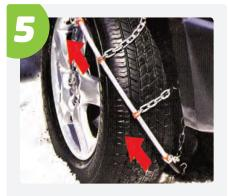
Start rolling both plastic hoops **anticlockwise** around the wheel. Rotate both plastic hoops together at the same time.
