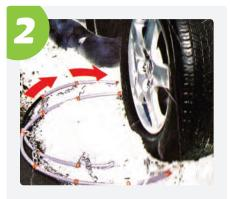
Place chains on the ground facing the wheel. Slide chains around behind the wheel.
