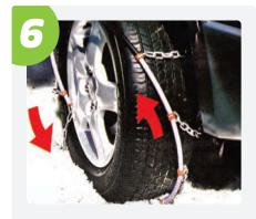
Keep rotating both plastic hoops around the wheel until the **black band** sits at the **top front** of the tyre.
