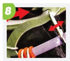
Tighten the ratchet and cam lever, once the chains are tight secure the lever under the **side loop** along with any excess chain. Move vehicle forward 10m and re-tighten the chains until **very tight**.
