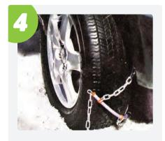
Lift the hook and chain around the wheel and connect together at the **top rear** of the tyre.
