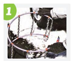
Hold chains up and remove any twists so they hang freely. Ensure the **black band** is on the bottom hoop with the open end facing the wheel.
