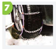
Shuffle the chains around the tyre so they sit squarely on the tyre and then tighten the chains around the wheel. Adjust the inside hook first **then the front lever.**
