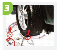
Locate the hook and chain at the end of the chain loops. These are marked with multi-coloured washers.
